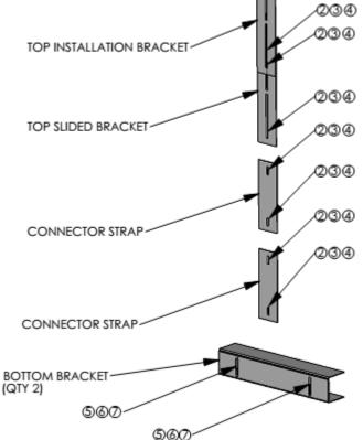
**STEP 1-** ALIGN TOP INSTALLATION BRACKET WITH REAR EDGE OF UPPER DRAWER FRAME. IF THIS BRACKET DOES NOT REACH THE DRAWER FRAME, ADD THE TOP SLIDER BRACKET AND ASSEMBLE WITH 2 SETS OF #8 SCREWS, NUTS, AND WASHERS (ITEMS #2, #3 & #4). ADJUST THESE 2 BRACKETS SO THAT, WHEN POSITIONED BEHIND DRAWER AND HOLES ARE ALIGNED, THE DRAWER HANGS LEVEL. SECURE THE TOP INSTALLATION BRACKET TO THE UNDER SIDE OF
