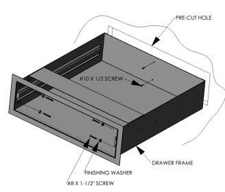
STEP 3- PLACE THE DRAWER FRAME INSIDE THE PRE-CUT HOLE IN THE FRONT OF THE ISLAND (PER CUT-OUT DIMENSIONS ON PAGE 4). CAREFULLY SLIDE THE FRAME ALL THE WAY IN UNTIL THE FRONT FLANGE IS FLUSH WITH THE ISLAND FRONT SURFACE. USE THE #8 X 1-1/2" SCREWS AND FINISHING WASHERS PROVIDED TO SECURE FRAME. IF FRONT SURFACE IS A HARD MATERIAL, IT MAY BE NECESSARY TO DRILL PILOT HOLES WITH A 1/8 TO 5/32 DRILL BIT.
