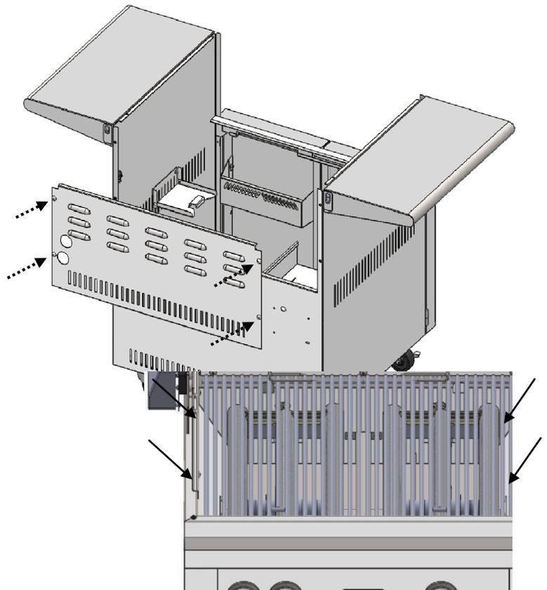
Once the grill has been placed inside the cart. You will want to remove the following screws and replace them with the supplied screws.
