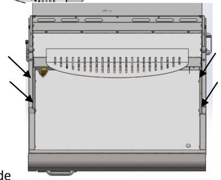
Once the grill has been placed inside the cart. You will want to remove the following screws and replace them with the supplied screws.
