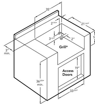
\* 2" round hole must be located at rear of grill cutout. 120V GFI outlet must be located within 6' of the 2" hole.
