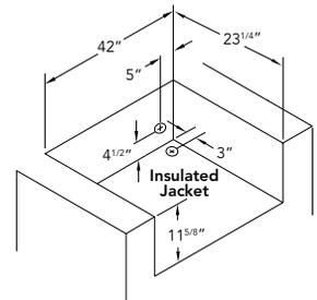
Note: Insulating jacket required for all grills installed into a combustible enclosure. For natural gas grills, Lynx recommends using 3/4" gas lines. Side burners may be rotated 90 degrees. See installation manuals for details.
